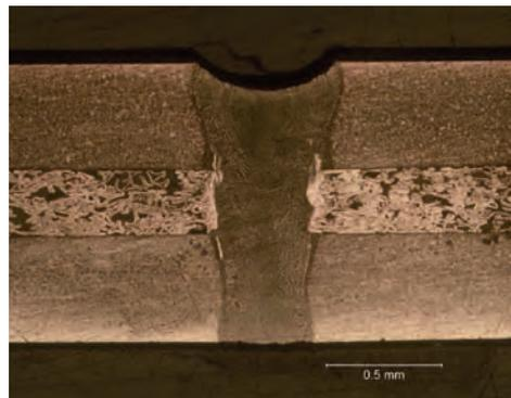
*Laser welding of nickel foam electrode tabs*
