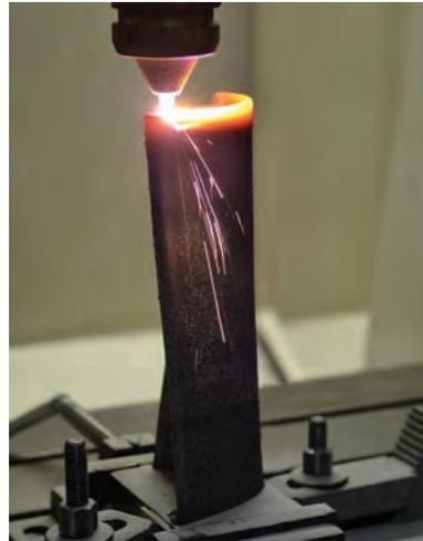
*Turbine blade demonstrator component built at CCL-L using laser based additive manufacturing*
