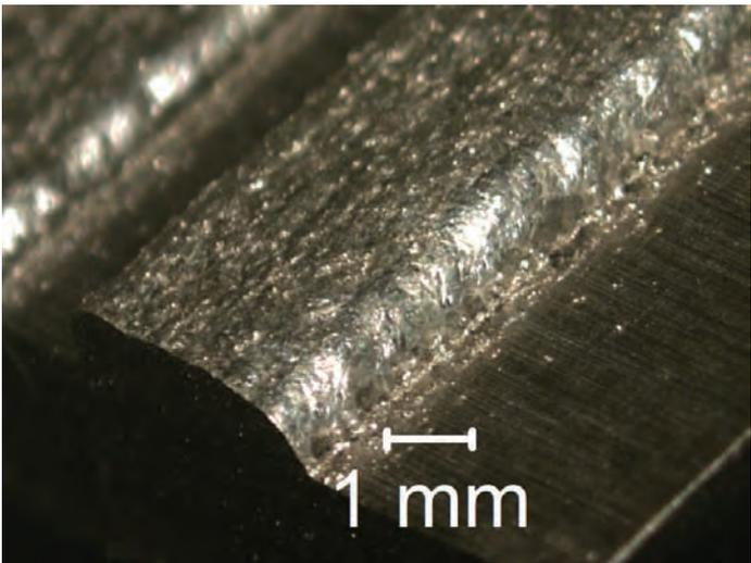
*Inconel 738 deposited on steel using MBLAM*
