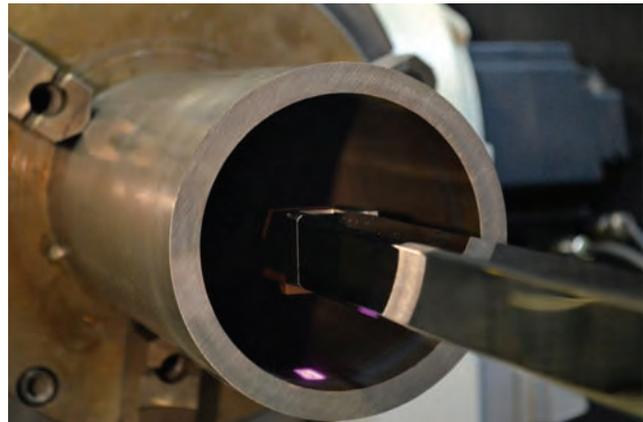
*New ID heat treatment head, developed by CCL-L in 2013*
