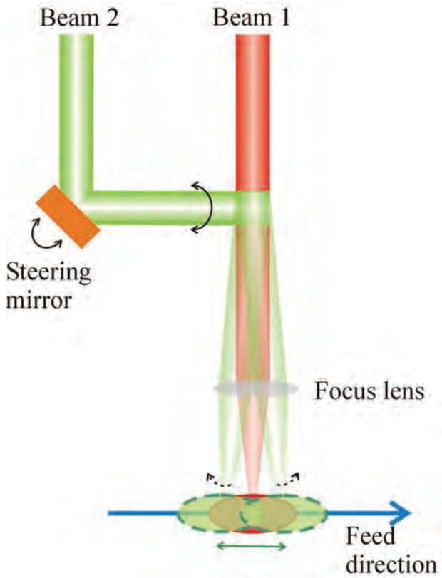
*Schematic of Multi-Beam LAM*
