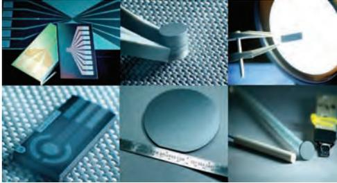
*Custom tailored boron-doped diamond electrodes for electrochemical applications*
