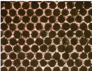
*Laser drilling of very high aspect-ratio holes in Tantalum*
