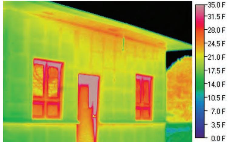
Thermal scan of a commercial building, retrofitted by Dow Corning, Dryvit and CSE using vacuum insulation panels (VIPs). The low surface temperature of the wall represents the thermal insulating capability of the new technology (blue and green representing lower, yellow and red representing higher, heat losses).
